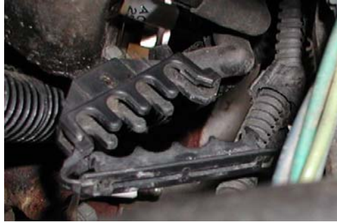
Figure 6: Ignition Wire Clamp located near Air Pump – F Body
