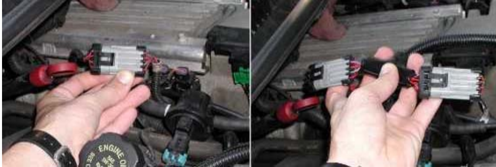
Figure 1: Opti-Spark Diagnostic Connectors – Before (left) and After (right) T-Harness Installation
